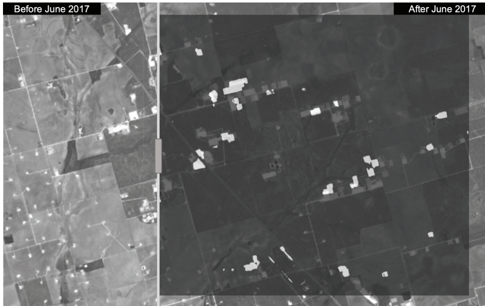
Figure 15.4 Automated change detection simplifies finding new development, as seen here around a wind farm in lesser prairie-chicken habitat in Texas in 2015. The change in surface reflectance (right, where bright white indicates change and dark is no-change in the overlay) is calculated from multi-band satellite imagery (left). A full explanation of the method, as well as dynamic figures with sliders to view changes, can be found at https://defenders-cci.org/analysis/LPC_delisting/ . Image source: public domain Sentinel-2 imagery from the European Space Agency.
