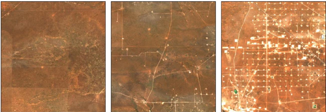
*Figure 4. Sentinel-2 satellite imagery collected during April – June, 2020 showing different levels of habitat fragmentation. Low (left), medium (center), and high (right) habitat fragmentation was measured as the distance of all habitat pixels to the nearest non-habitat pixel.*
